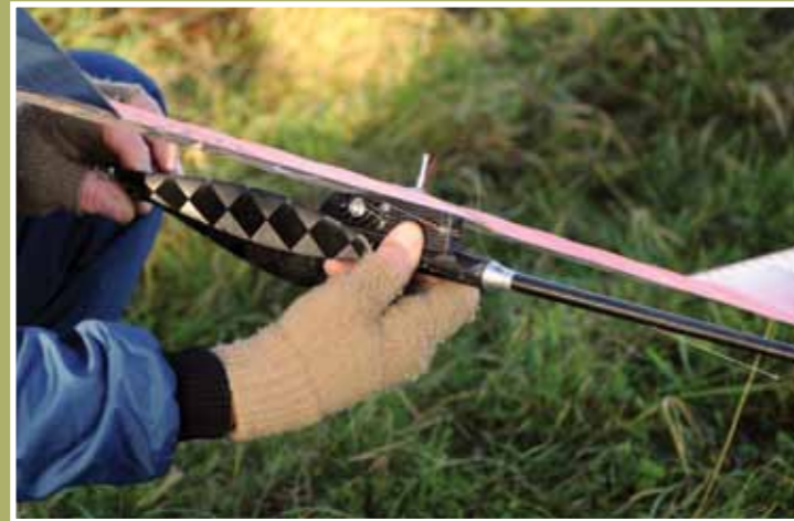
Right: Pete Brown was flying this very modern model. Note spectacular carbon blades - the fine bent wire is the tracker aerial. Carbon boom fitted to motor tube by very neat aluminium turning.
