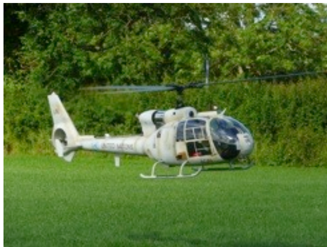
Ian Bishop's Cine Scale Gazette powered by a JetCat Pht3 turbine
